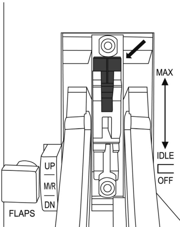
(In this position, the AFTERBURNER stop is disabled)
