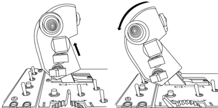
To power the motors back on, simply push the throttle levers forward (and then slightly down), into the IDLE position.
