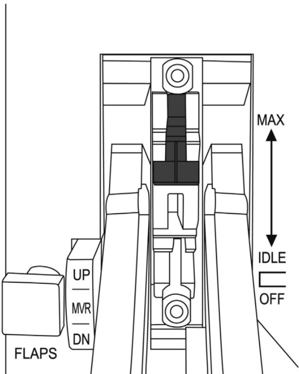
(In this position, the AFTERBURNER stop is now enabled)
